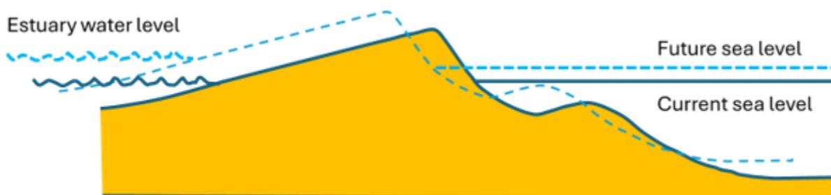
**Figure 4-5 Schematic of landward and upward shift in entrance berm profile due to sea level rise (Streamology 2022b)**
