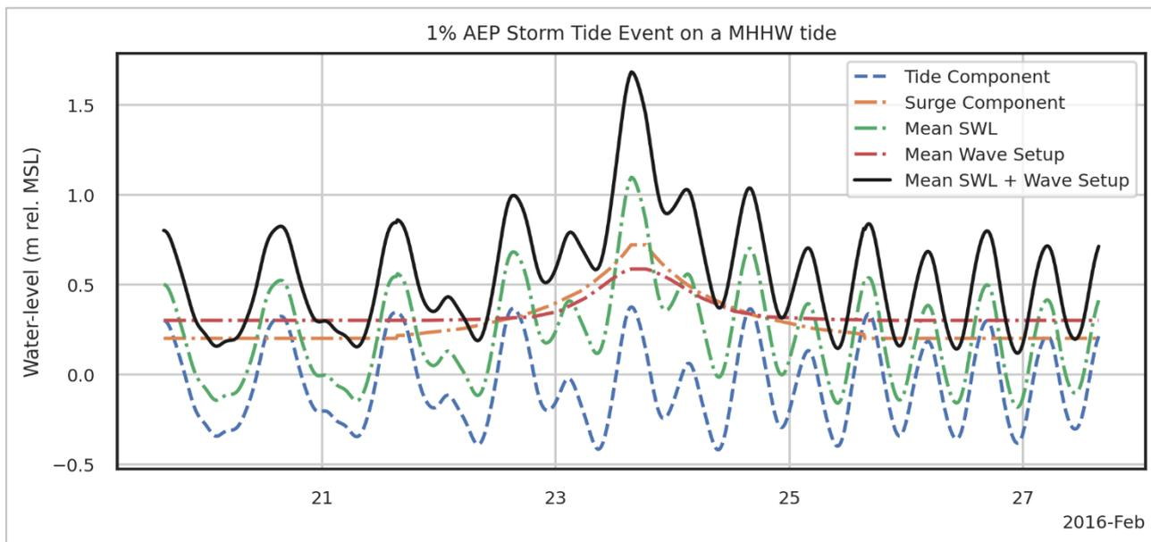
**Figure 4-4 1% AEP storm tide time series**
