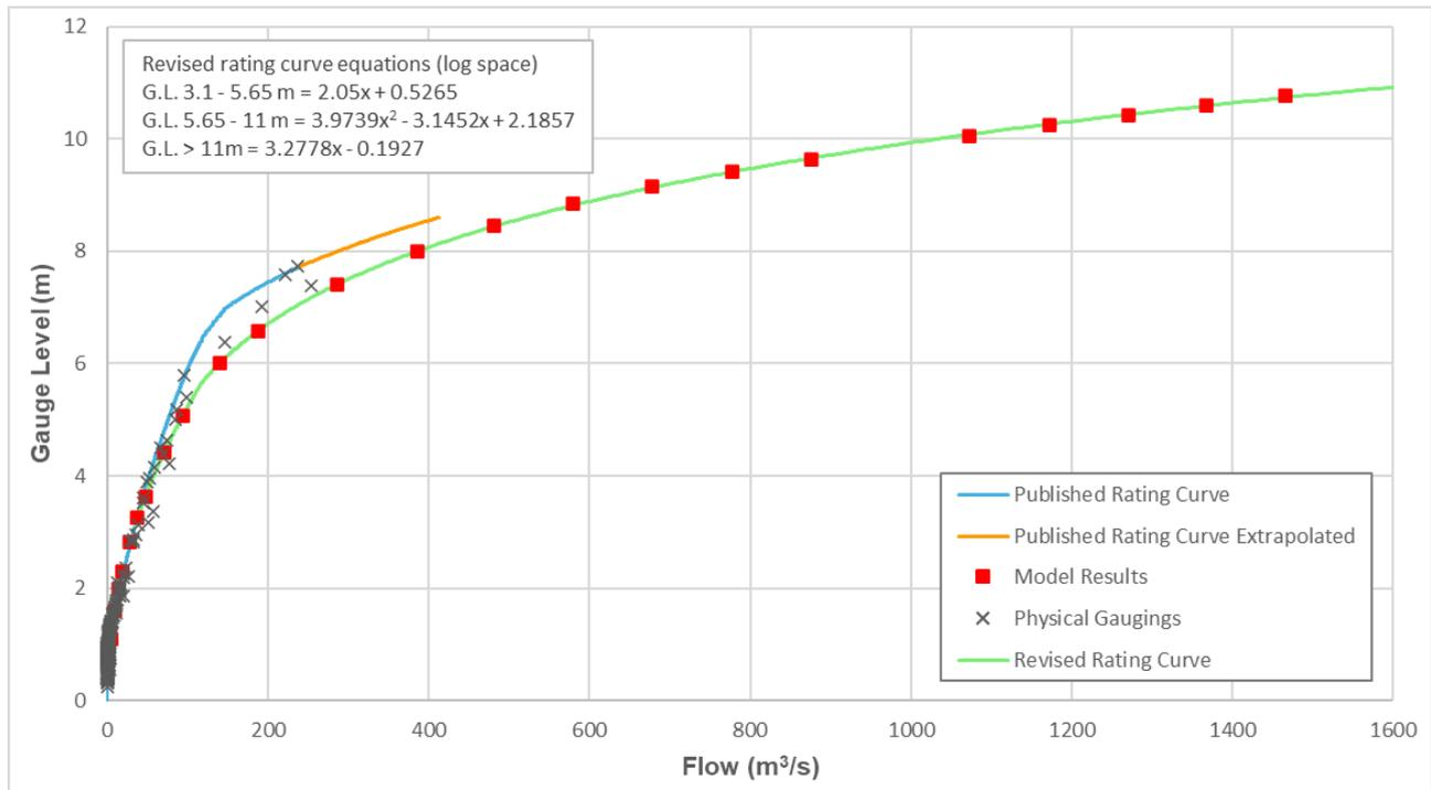
**Figure 3-2 Merri River at Woodford rating curve verification**
