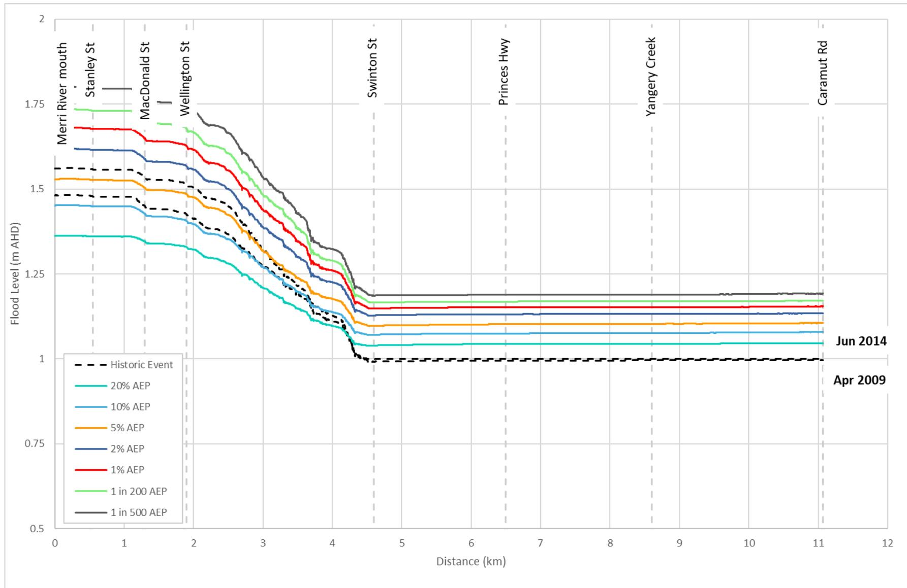
Figure 5-5 Storm tide event flood level long-section
